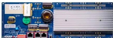
BS485 Communication between battery and inverters Band rate:9600bps BS485 Interface Communication between powerlib packs of BMS and PC Band rate:9600bps
