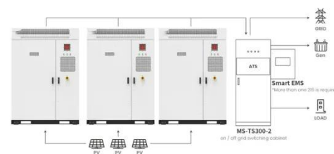
Application scenarios of energy storage battery products
