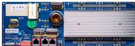
RS485 Communication between battery and inverters Band rate:9600bps RS485 Interface Communication between parallel packs or EMS and PC Band rate:9600bps
